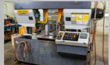
HydMech 14A dual-column automatic band saw
