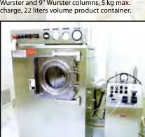
STOKES 42 Sq. Ft. Heresite Lined Vacuum Shelf Dryer, (7) 2' x 3' shelves, available with Sihi vacuum pump and heating unit at additional cost.
