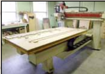
PHOENIX RG-48 XHDR Bridge Type CNC Router, 4' x 8' table
