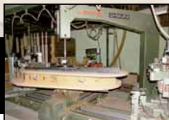
SHIMURA NRC-2200WT-C Overhead Production Router/Shaper
