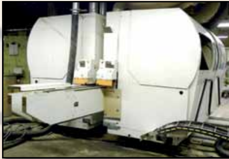
2003 SCMI Concept 2000 CNC Double End Tenoner, sn AA1/013368, w/SCMI Concept 454D control, sn 2638485048F, (8) drives per side
