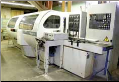
2003 SCMI Topset 23 Molder, sn AA1/011948, 6-head w/BEN-200 feeder, sn MA/003556
