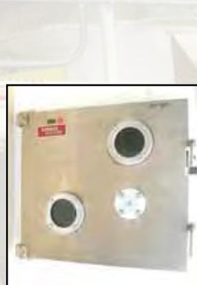
**STOKES 42 Sq. Ft. Heresite Lined Vacuum Shelf Dryer**, (7) 2' x 3' shelves, available with Sihu vacuum pump and heating unit at additional cost.
