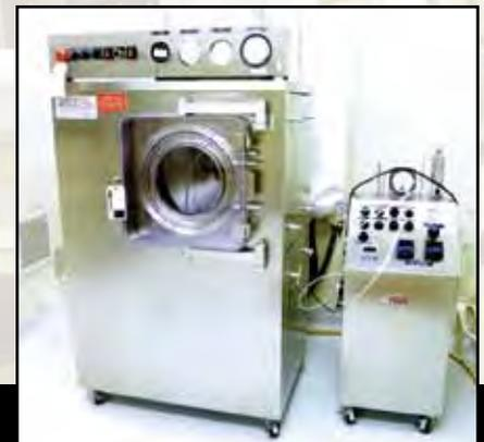
**THOMAS ENGINEERING 24" Accela-Cota**, Mdl. 24-V, S/S coating pan, 24" diameter perforated pan.
