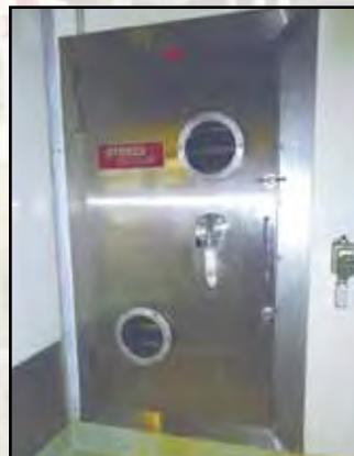
**STOKES 90 Sq. Ft. Stainless Steel Vacuum Shelf Dryer**, (15) 2' x 3' S/S shelves, rated 50 PSI/full vacuum @ 650° F, steam heat, Mdl. 438F15, S/N 73639, available w/vacuum skid and heat transfer unit at additional cost.
